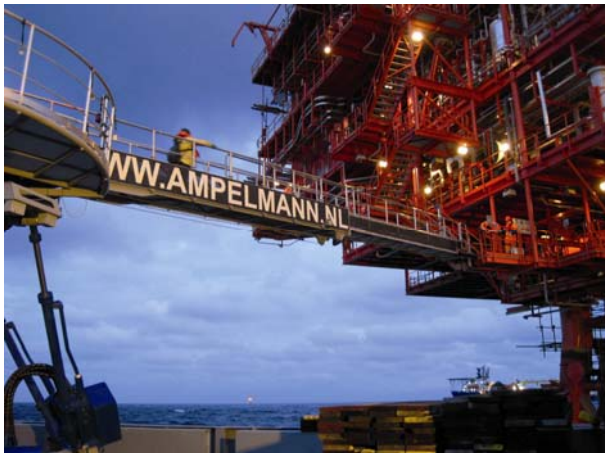
Ampelmann gangway for personnel safe access to offshore platform.
